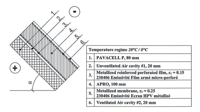
Figure 1. Roof construction design
